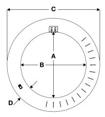
Representative sticker provided with retrofit lamps which must be affixed to the luminaire in order to maintain the UL rating of the luminaire after retrofit when wiring directly to line voltage. In the event lamps are used at Type A with a compatible ballast, retain the stickers for future retrofit compliance.
